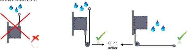
4. The wire should not be pulled in angular. If needed, please use guide rollers.
