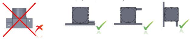
3. If there is the possibility of splashing of water (like rain) on the device, the wire outlet must not look upwards. If the wire needs to go upwards, please use guide rollers.
