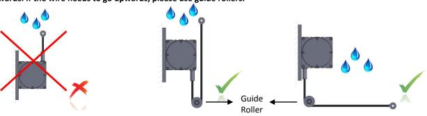
4. The wire should not be pulled with an angle. If needed, please use guide rollers.
