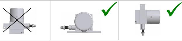
3. If there is a trickle of water (like a rain), the wire outlet must not be a drip of water upstream. If needed please use guide rollers.
