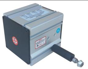
The AWP220 series are wire potentiometric position transducers that turn a linear motion into a resistance variation. They are made of a precision rotating potentiometer operated by a, winding or unwinding, stainless steel wire. Optionally other stroke lengths, cable length and socket connector can be requested.
