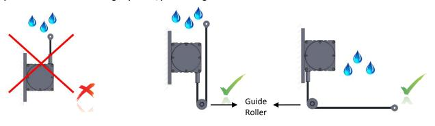
4. The wire should not be pulled with an angle. If needed, please use guide rollers.
