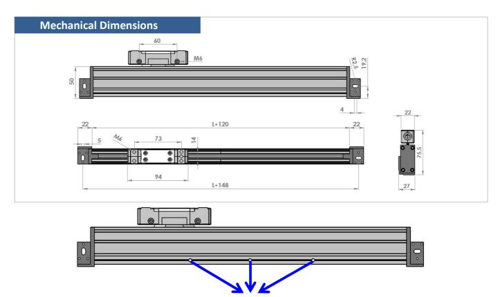
For long scale installations, generally it is not enough to fix the scale in 2 ends. In such cases, mounting holes can be opened over the lowest line on the ruler profile. Mounting holes can be opened from the desired location along the line with a diameter of 6 mm. Thus, long rulers can be secured in a healthy way.
