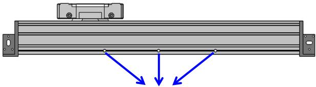
For long scale installations, generally it is not enough to fix the scale in 2 ends. To make a better fixing please make mounting holes the bottom line of the profile. You can make holes any point on the bottom line.
