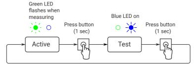
Illustration 3: Switching between active and test mode.
