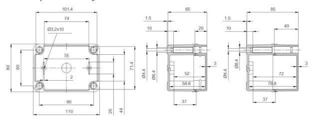
Illustration 6: Housing dimensions (in mm). Note: Drawing not including air inlet.
