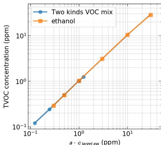
**Figure 4** TVOC concentration versus target gas set concentration times the relative response factor  $a$  (see **Table 6**), measured for two different target gases: (a) ethanol and (b) the two kinds of VOC mix, which is according to ISO16000-29:2014(E)<sup>10</sup> the most suitable proxy for TVOC.
