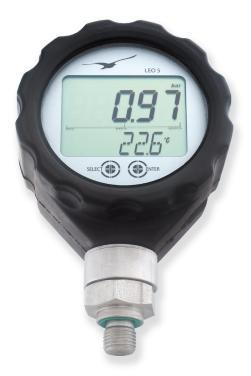
LEO 5 manometer accessories Rubber cover (shown above), transport case, belt pouch, spare batteries, various pressure adapters
